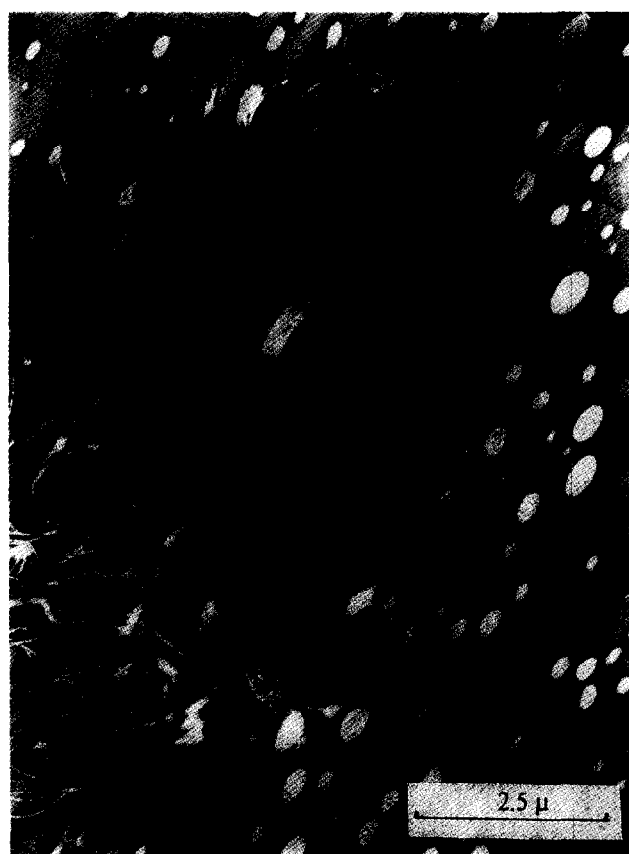
Figure 10 TEM micrograph of an 80/20 PC/PBT blend melted for 2 min at 260°C, quickly cooled ( 150^\circ\text{Cmin}^{-1} ) to 200°C and crystallized at that temperature for 8 min before quenching in iced water
