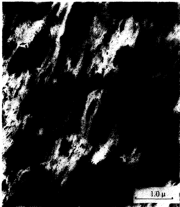
Figure 11 TEM micrograph of a 20/80 PC/PBT blend melted for 2 min at 260^\circ\text{C} , quickly cooled ( 150^\circ\text{C min}^{-1} ) to 200^\circ\text{C} and crystallized at that temperature for 60 min before quenching in iced water
