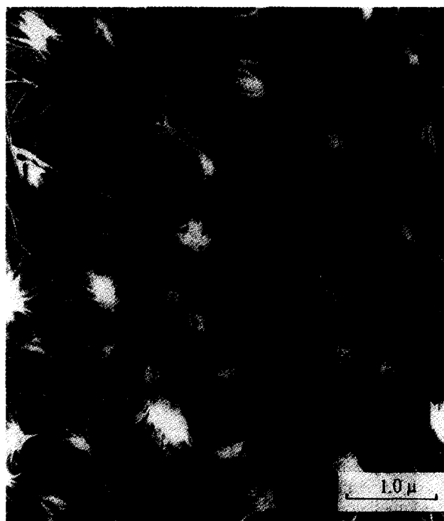
Figure 9 TEM micrograph of an 80/20 PC/PBT blend melted for 2 min at 260°C, quickly cooled ( 150^\circ\text{Cmin}^{-1} ) to 200°C and crystallized at that temperature for 60 min before quenching in iced water
