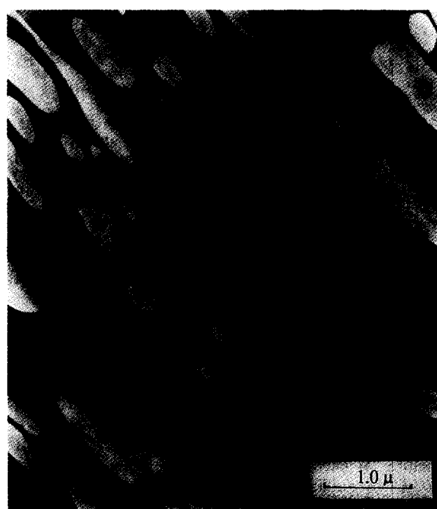
Figure 5 TEM micrograph of a 60/40 PC/PBT blend after melting for 2 min at 260°C then quenching in iced water
