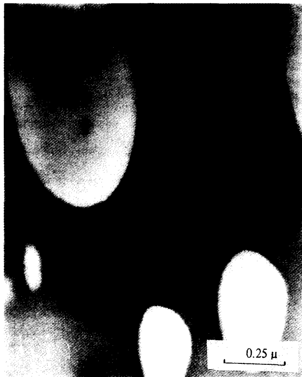
Figure 25 TEM micrograph (high magnification) of an 80/20 PC/PBT blend melted for 2 min at 260°C, quickly cooled ( 150^{\circ}\text{C min}^{-1} ) to 150°C and annealed at that temperature for 10 min before quenching in iced water
