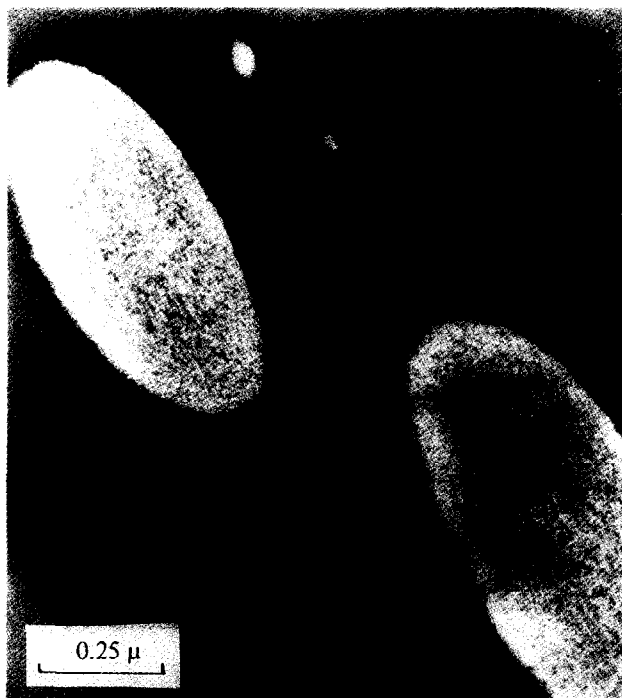
Figure 26 TEM micrograph (high magnification) of an 80/20 PC/PBT blend melted for 2 min at 260°C, quickly cooled ( 150^{\circ}\text{C min}^{-1} ) to 105°C and annealed at that temperature for 10 min before quenching in iced water
