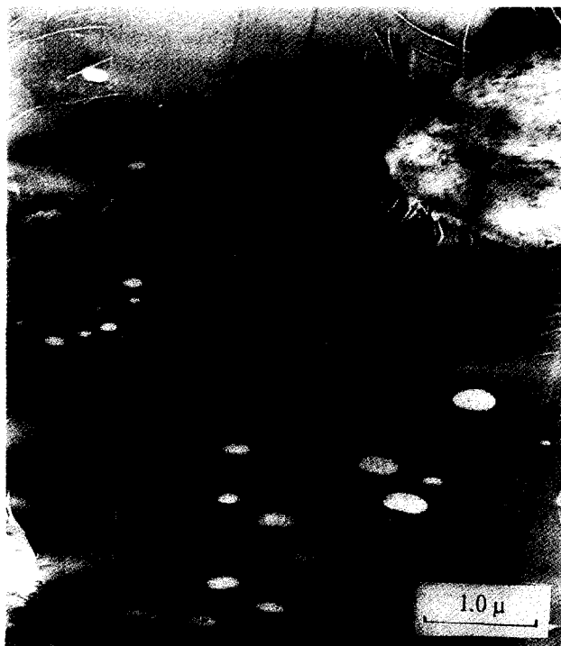
Figure 13 TEM micrograph of a 60/40 PC/PBT blend melted for 2 min at 260^\circ\text{C} , quickly cooled ( 150^\circ\text{C min}^{-1} ) to 200^\circ\text{C} and crystallized at that temperature for 2 min before quenching in iced water
