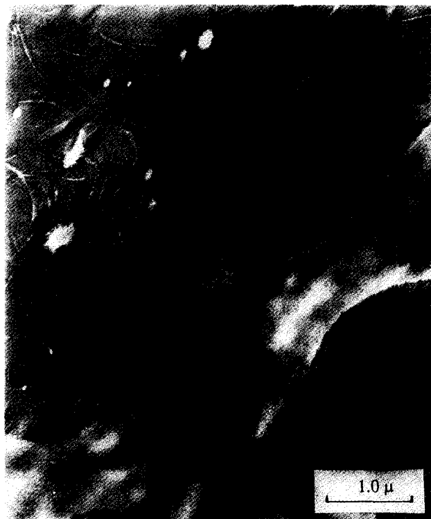
Figure 12 TEM micrograph of a 60/40 PC/PBT blend melted for 2 min at 260^\circ\text{C} , quickly cooled ( 150^\circ\text{C min}^{-1} ) to 180^\circ\text{C} and crystallized at that temperature for 15 min before quenching in iced water
